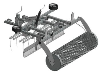
finishes the surface. The harrow also has side wheels that enable working along walls with no damage. Easily made adjustments enable weight and balance adjustments between the spring tines and roller/spreader assembly. Height adjustments to enhance processing difficult soils are made quickly and easily.
